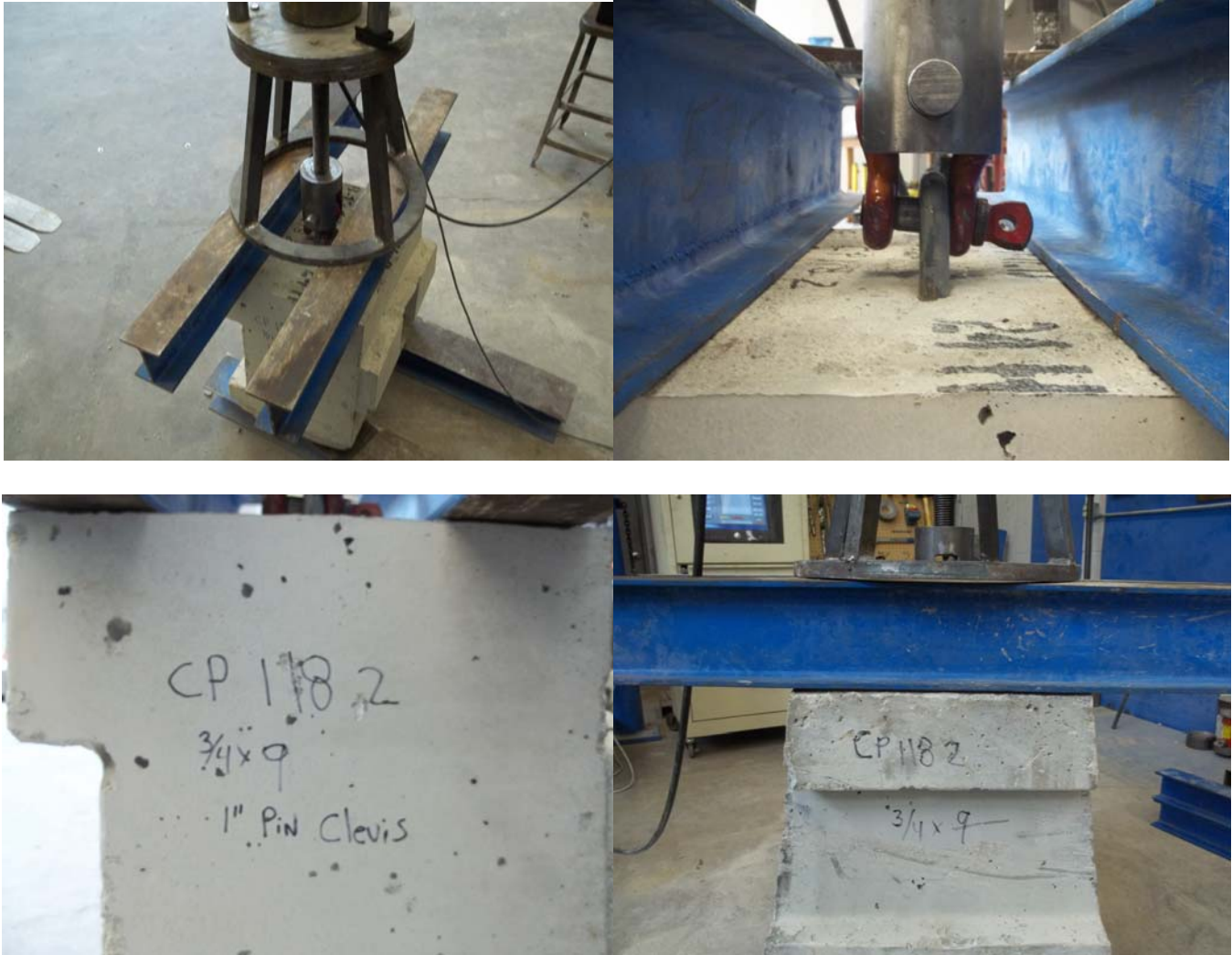
Figure 1 – 90-degree Tension Test Set-up
