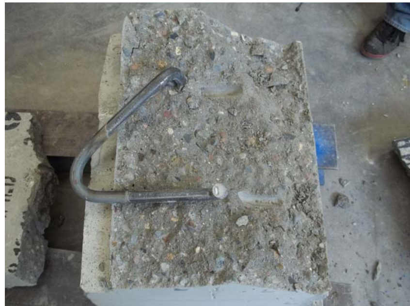
Figure 2 – Tension Failure Mode
